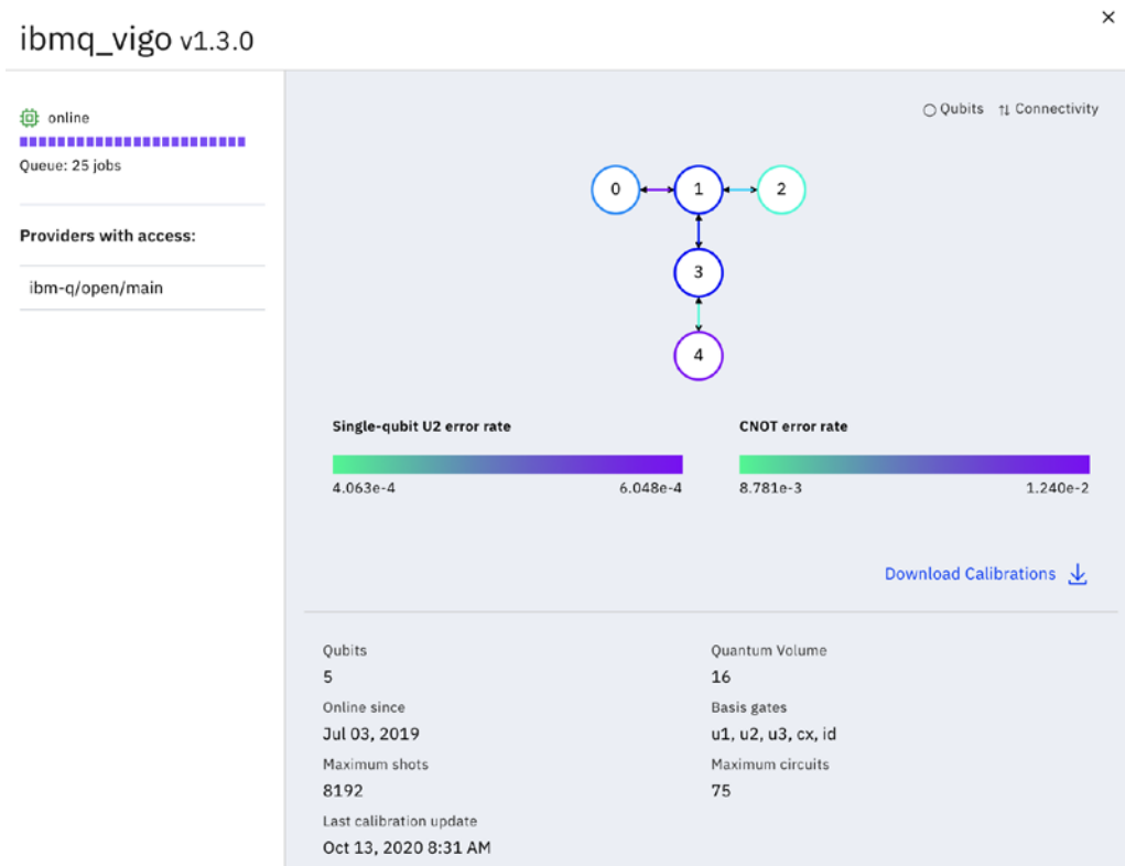
Figure 8.6 – Details of the ibmq_vigo backend
